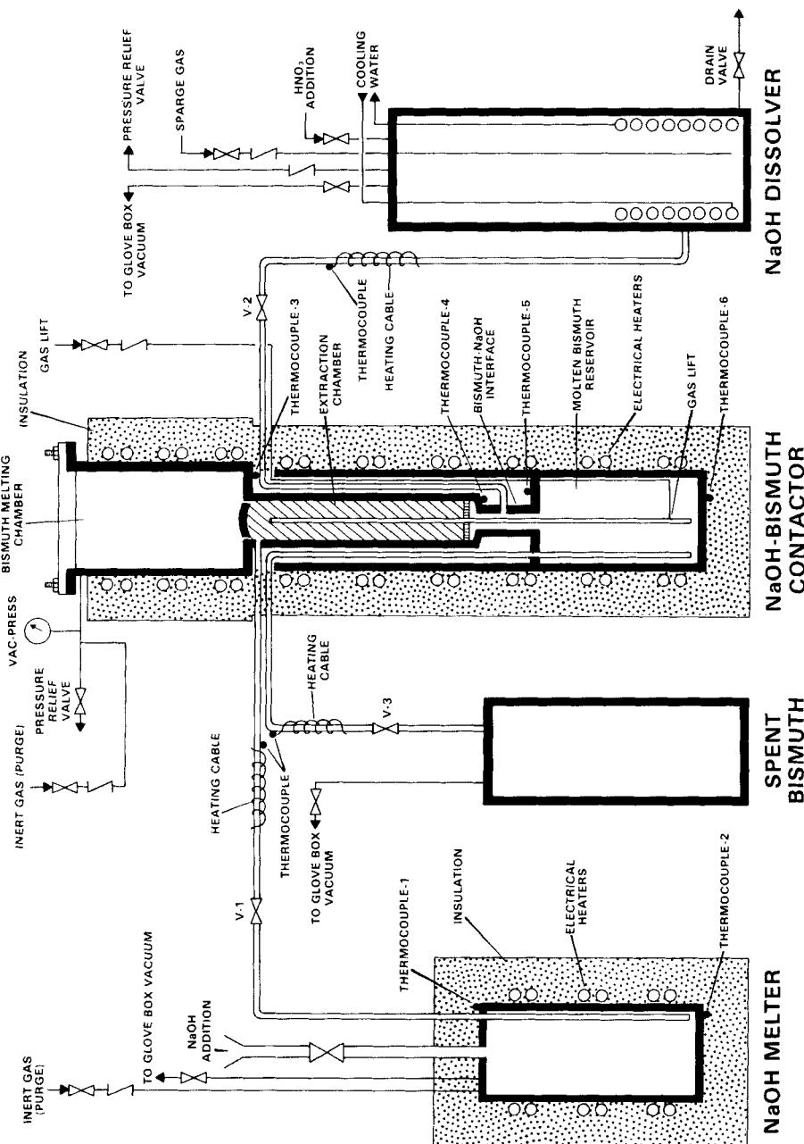
FIGURE 1: A Schematic View of the Pyrochemical Extraction Equipment
